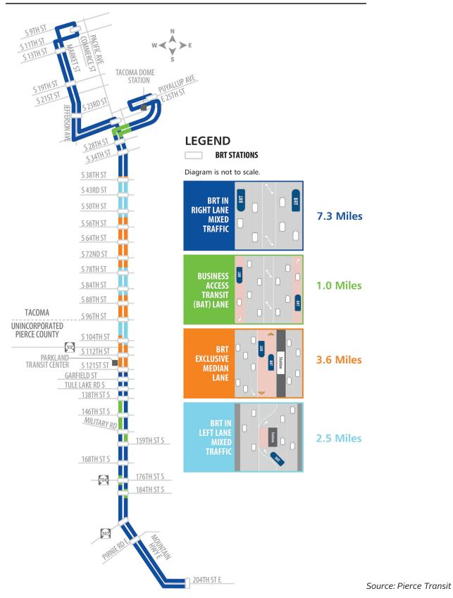
Figure 1-3: BRT Station Concept
