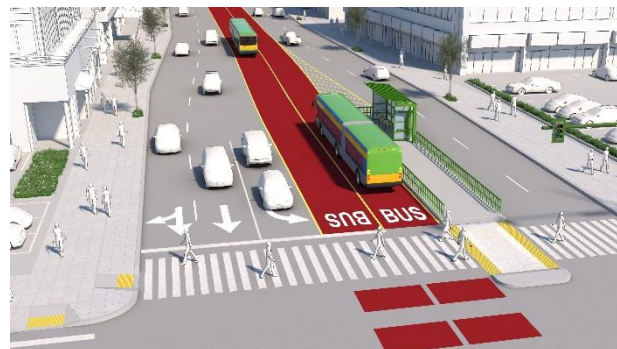
Median Exclusive Lane: Right Side Vehicle Boarding
