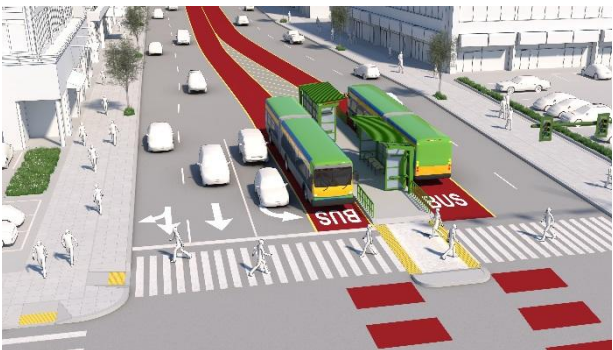
Median Exclusive Lane: Left Side Vehicle Boarding
