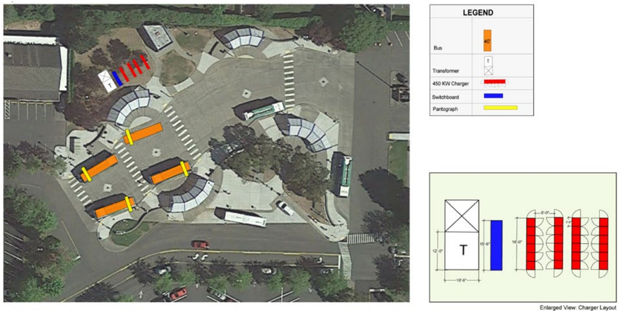
Figure 12: BEB Charging Layout at Lakewood Transit Center
