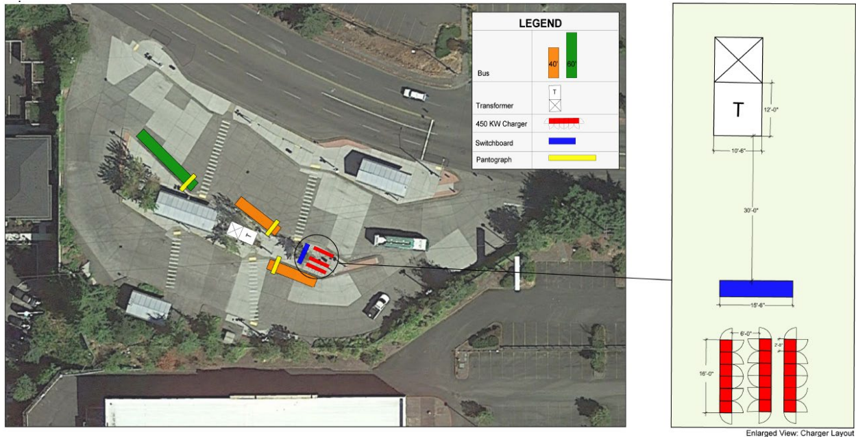
Figure 27: Tacoma Mall Electric Bus Charging – Option A
