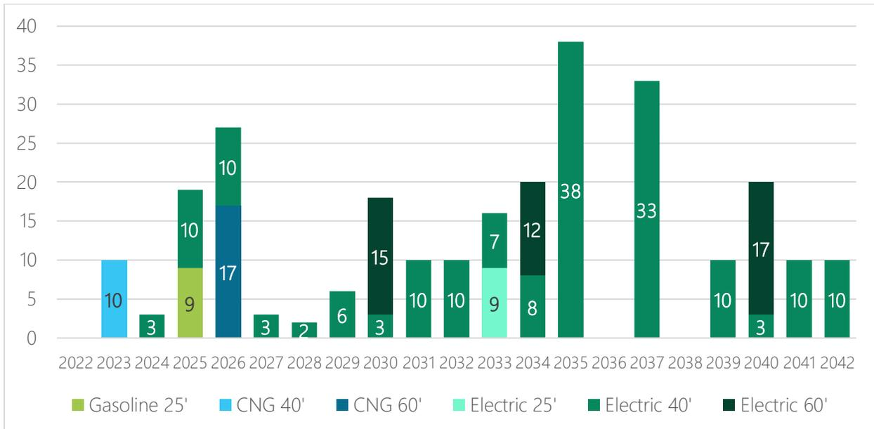
In order to operate BEBs, additional charging infrastructure will be required incrementally. Pierce Transit would primarily use 150 kW depot chargers to charge buses; however, a few on route chargers are needed once the fleet exceeds 18 BEBs. The charging infrastructure deployment will need to be completed by the time the buses arrive, so planning, design, and construction will need to occur prior to the deployment.
