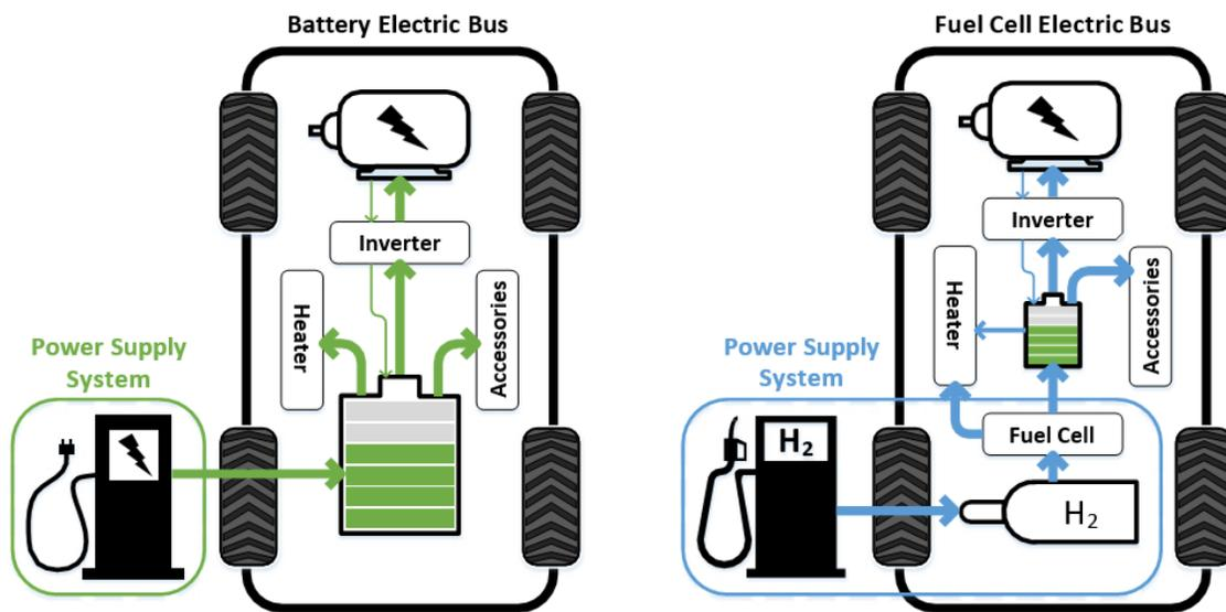
Figure 1: Battery Electric and Fuel Cell Bus Technologies
