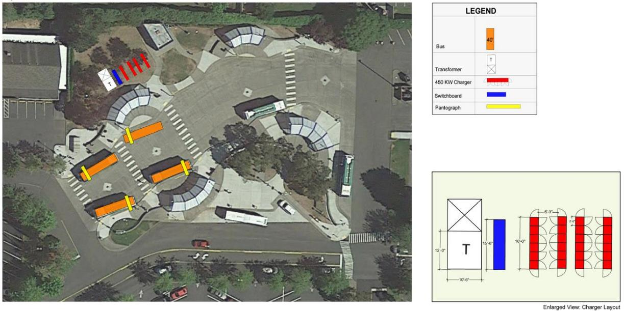
Figure 22: Lakewood Electric Bus Charging Aerial View - Option B
