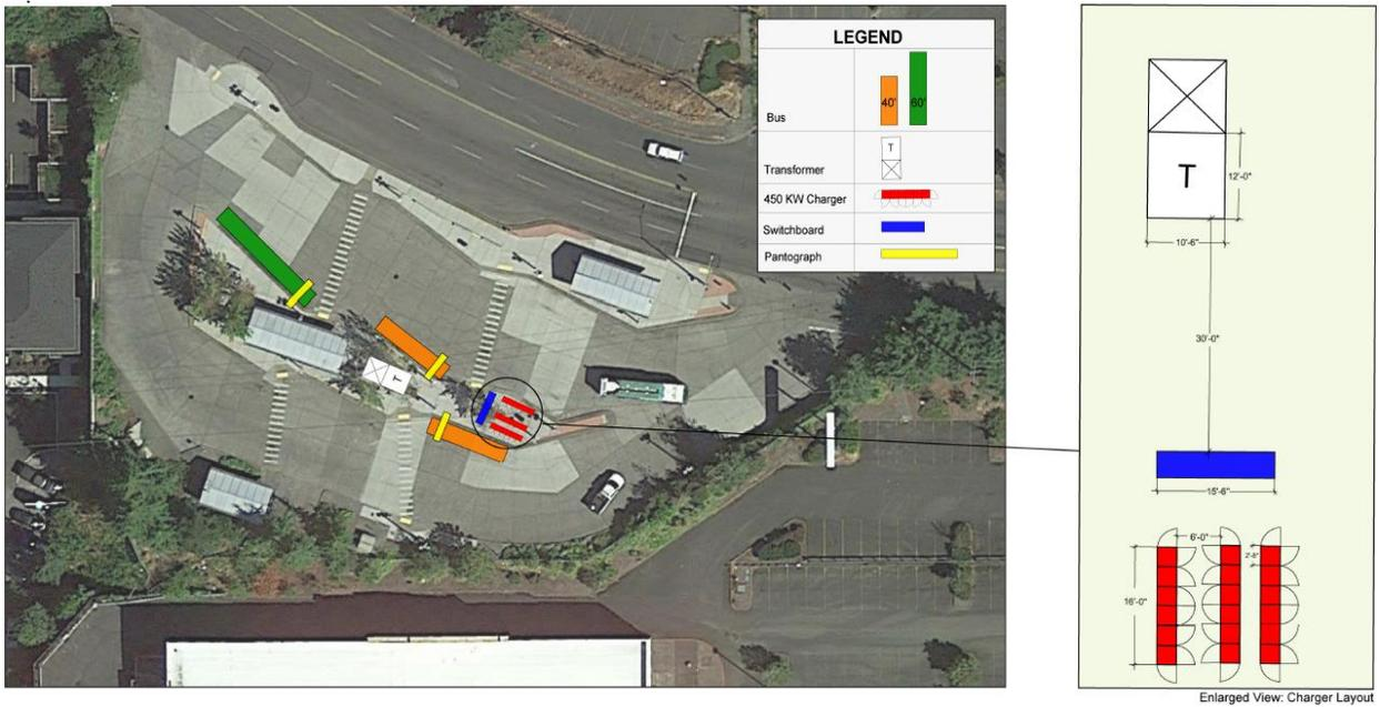
Figure 28: Tacoma Mall Electric Bus Charging – Option B
